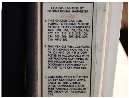
FIGURE 40. Test Vehicle Manufacturer's Label
