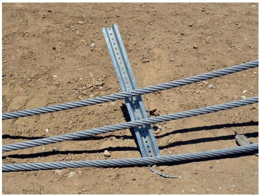
FIGURE 49. Test Article, Post-Test Damage
