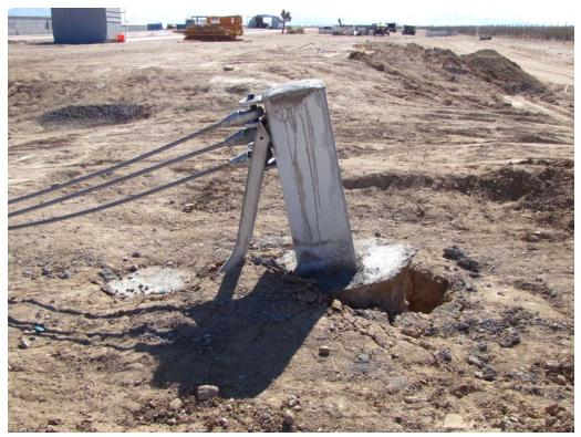
FIGURE 33. Test Article, Post-Test Damage
