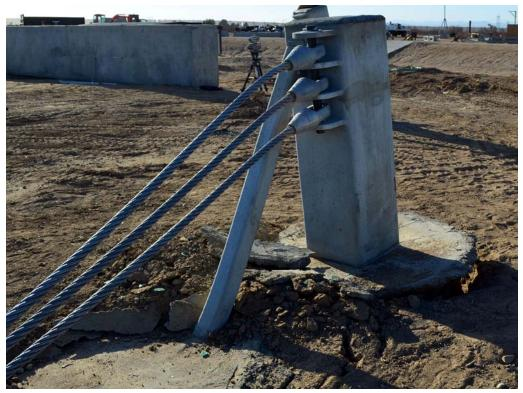
FIGURE 39. Test Article, Post-Test Damage
