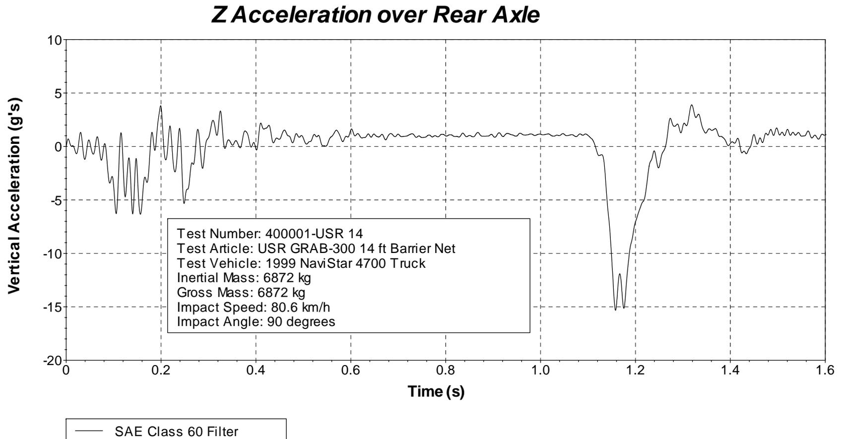
Figure 25. Vehicle vertical accelerometer trace for test 400001-USR14 (accelerometer located over rear axle).
