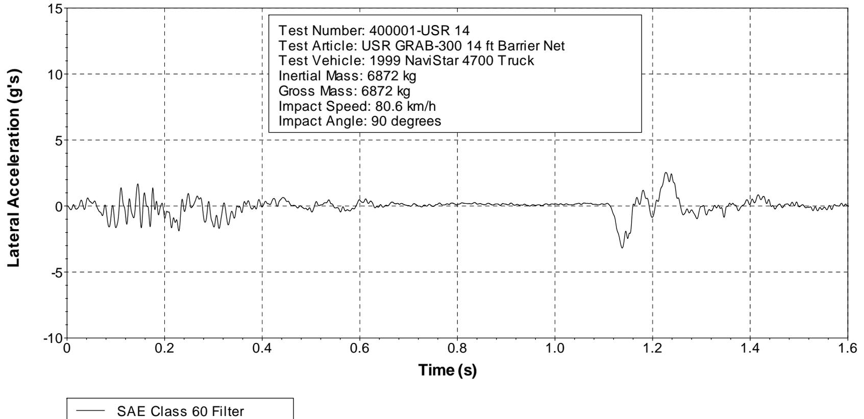
Figure 24. Vehicle lateral accelerometer trace for test 400001-USR14 (accelerometer located over rear axle).
