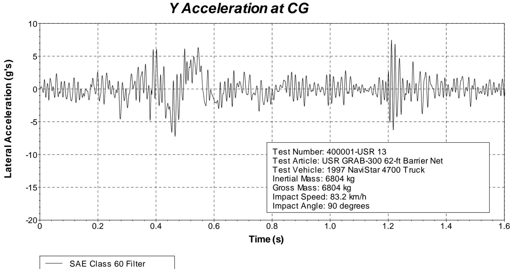
Figure 21. Vehicle lateral accelerometer trace for test 400001-USR13 (accelerometer located at center of gravity).
