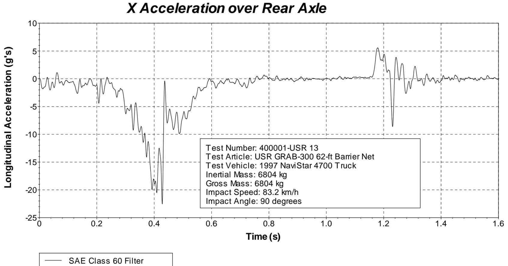
Figure 23. Vehicle longitudinal accelerometer trace for test 400001-USR13 (accelerometer located over rear axle).
