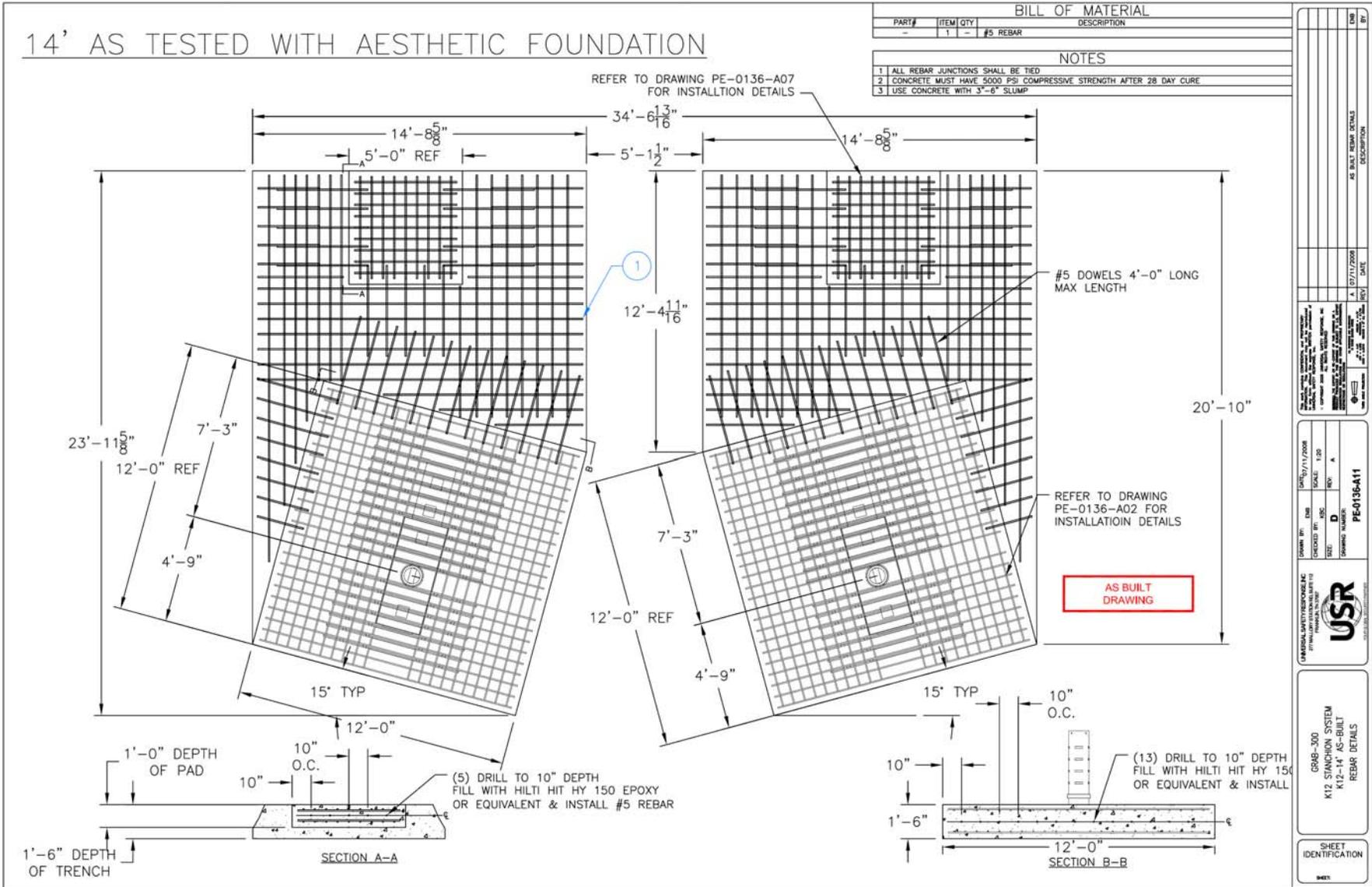
Figure 9. Details of the GRAB-300 14-ft barrier net – stanchion system rebar details.
