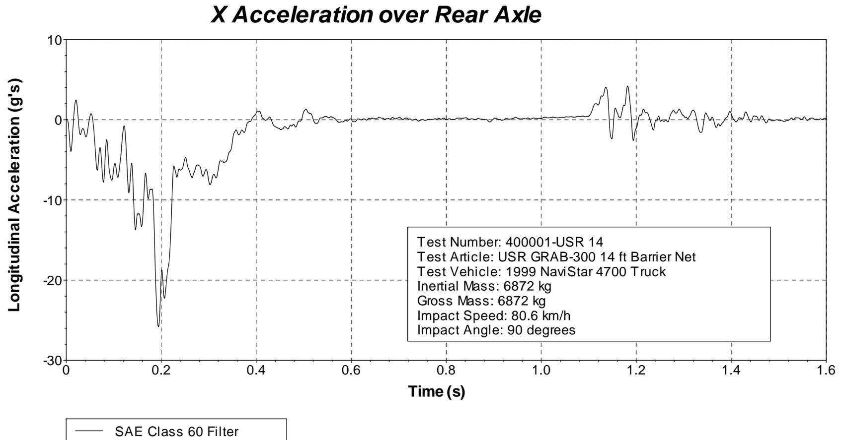
Figure 23. Vehicle longitudinal accelerometer trace for test 400001-USR14 (accelerometer located over rear axle).
