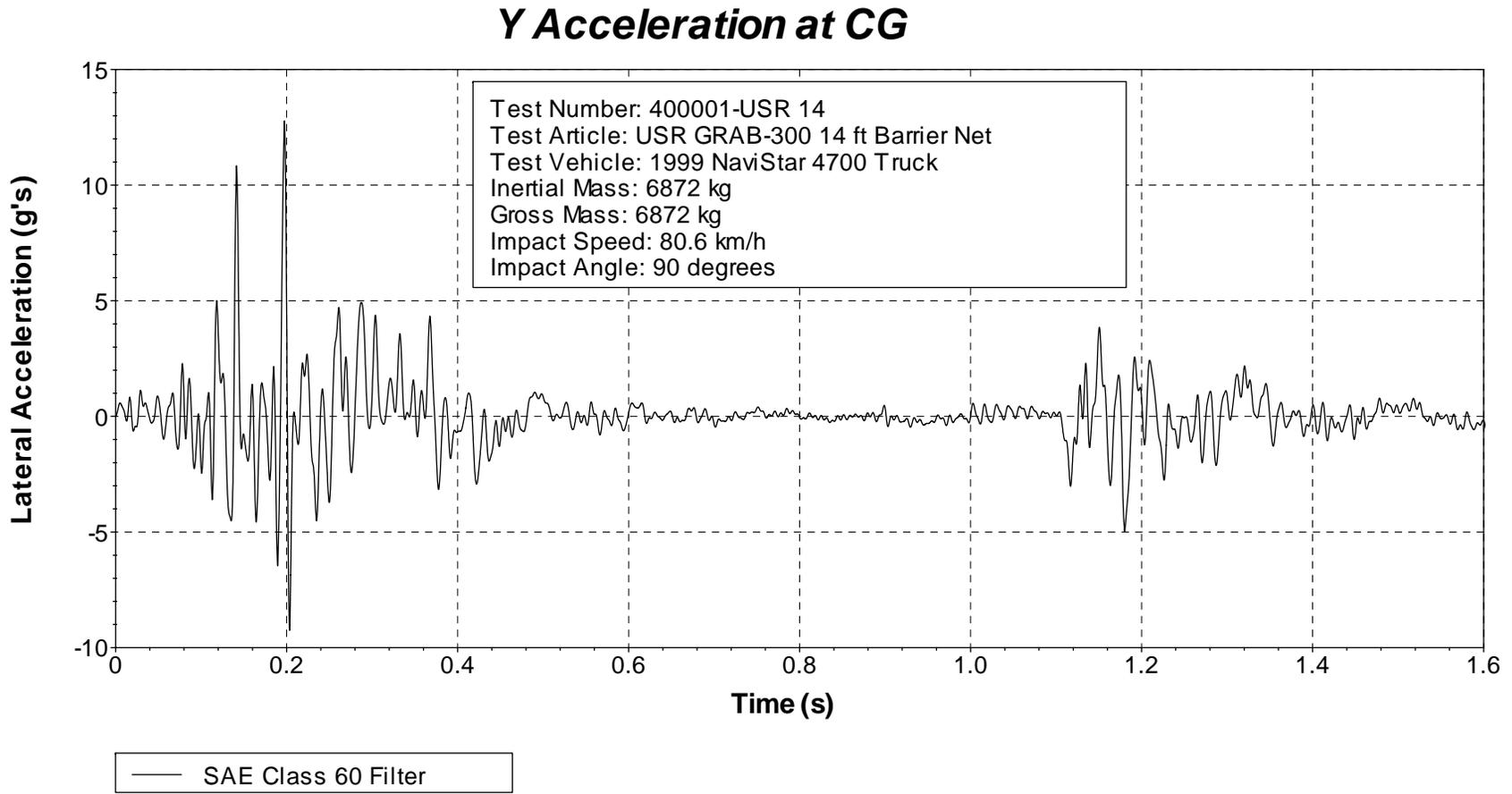
Figure 21. Vehicle lateral accelerometer trace for test 400001-USR14 (accelerometer located at center of gravity).
