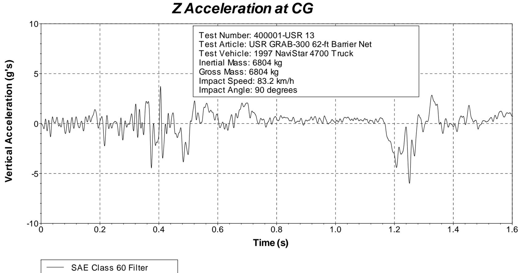
Figure 22. Vehicle vertical accelerometer trace for test 400001-USR13 (accelerometer located at center of gravity).
