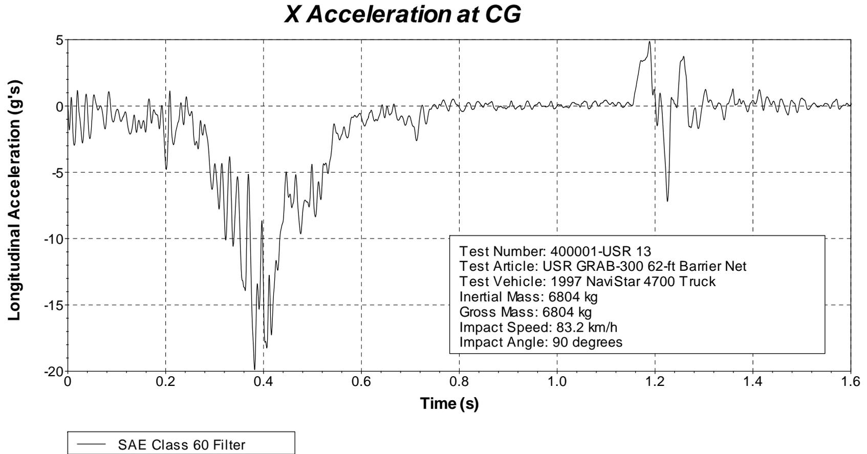
Figure 20. Vehicle longitudinal accelerometer trace for test 400001-USR13 (accelerometer located at center of gravity).
