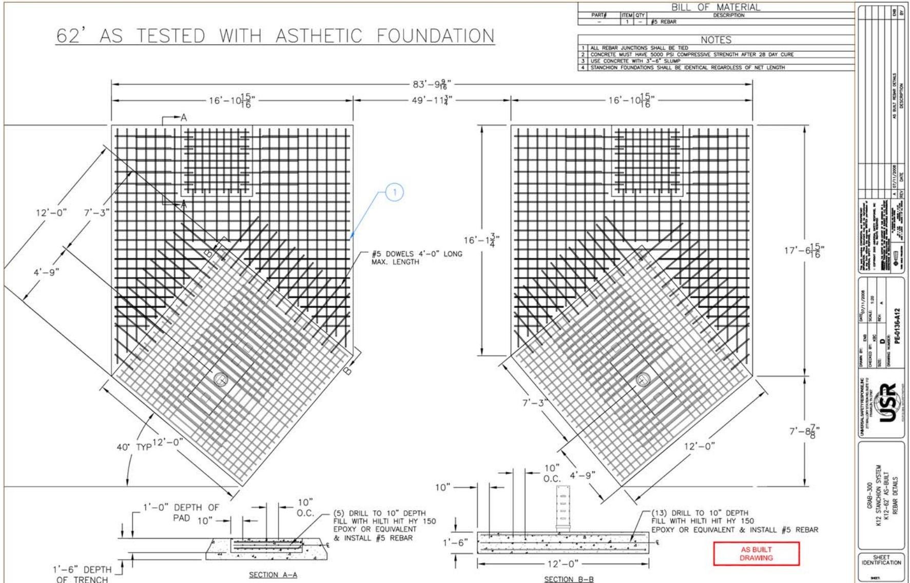
Figure 9. Details of the GRAB-300 62-ft barrier net – stanchion system rebar details..
