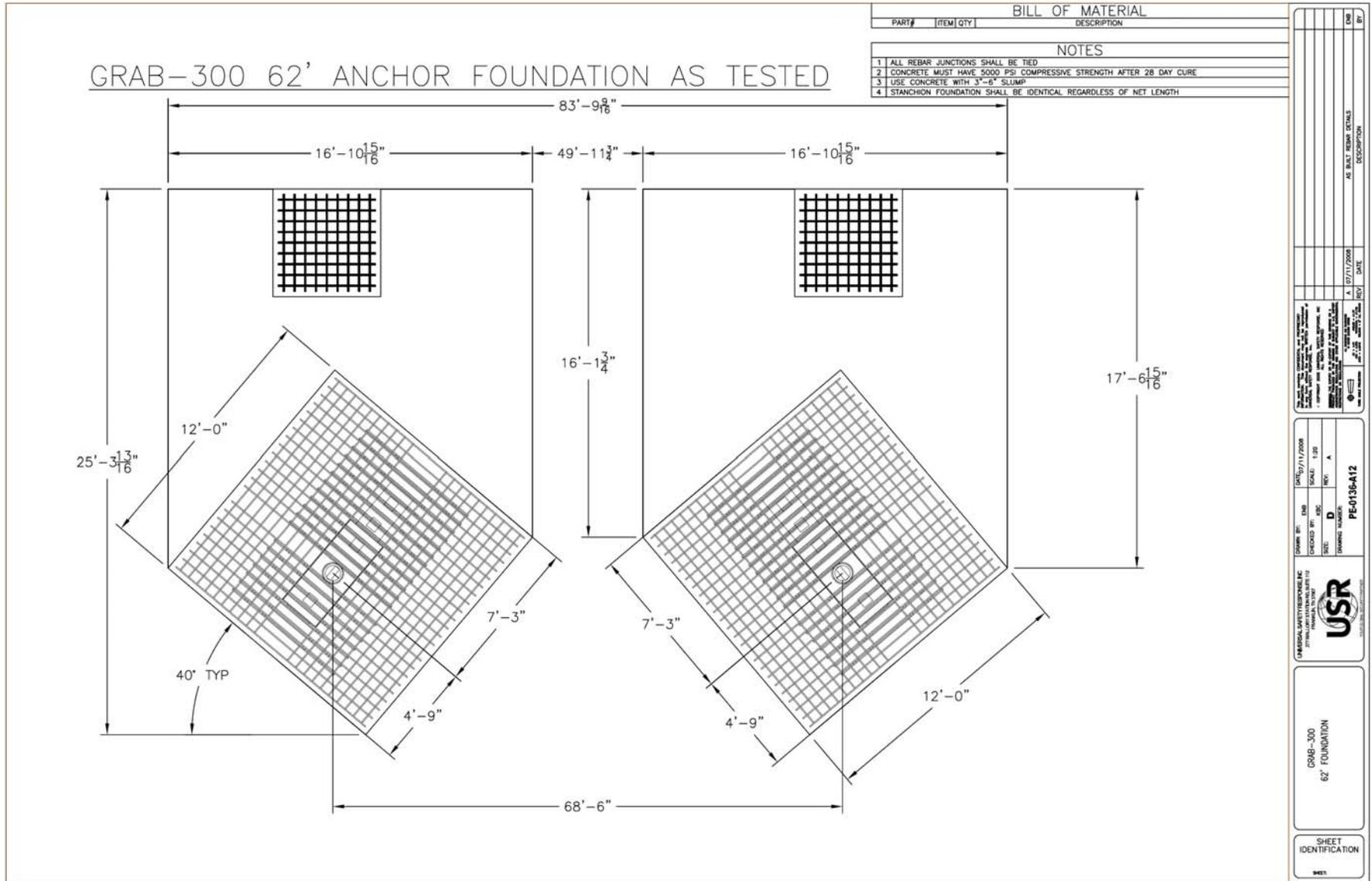
Figure 8. Details of the GRAB-300 62-ft barrier net – anchor foundation.
