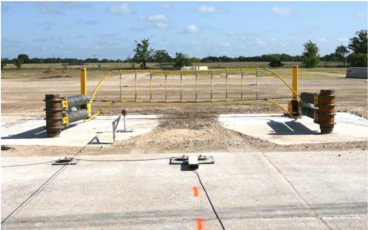
Figure 10. GRAB-300 14-ft barrier net prior to testing.
