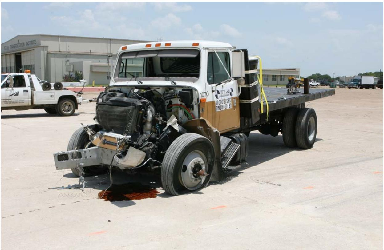
Figure 15. Vehicle after test 400001-USR13.
