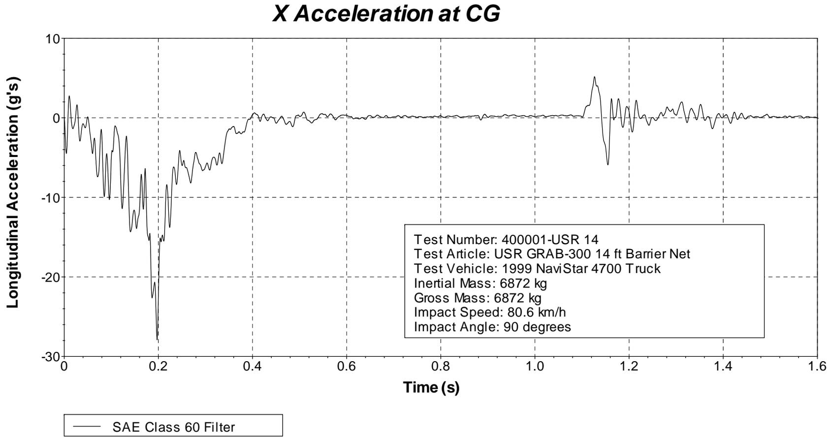
Figure 20. Vehicle longitudinal accelerometer trace for test 400001-USR14 (accelerometer located at center of gravity).
