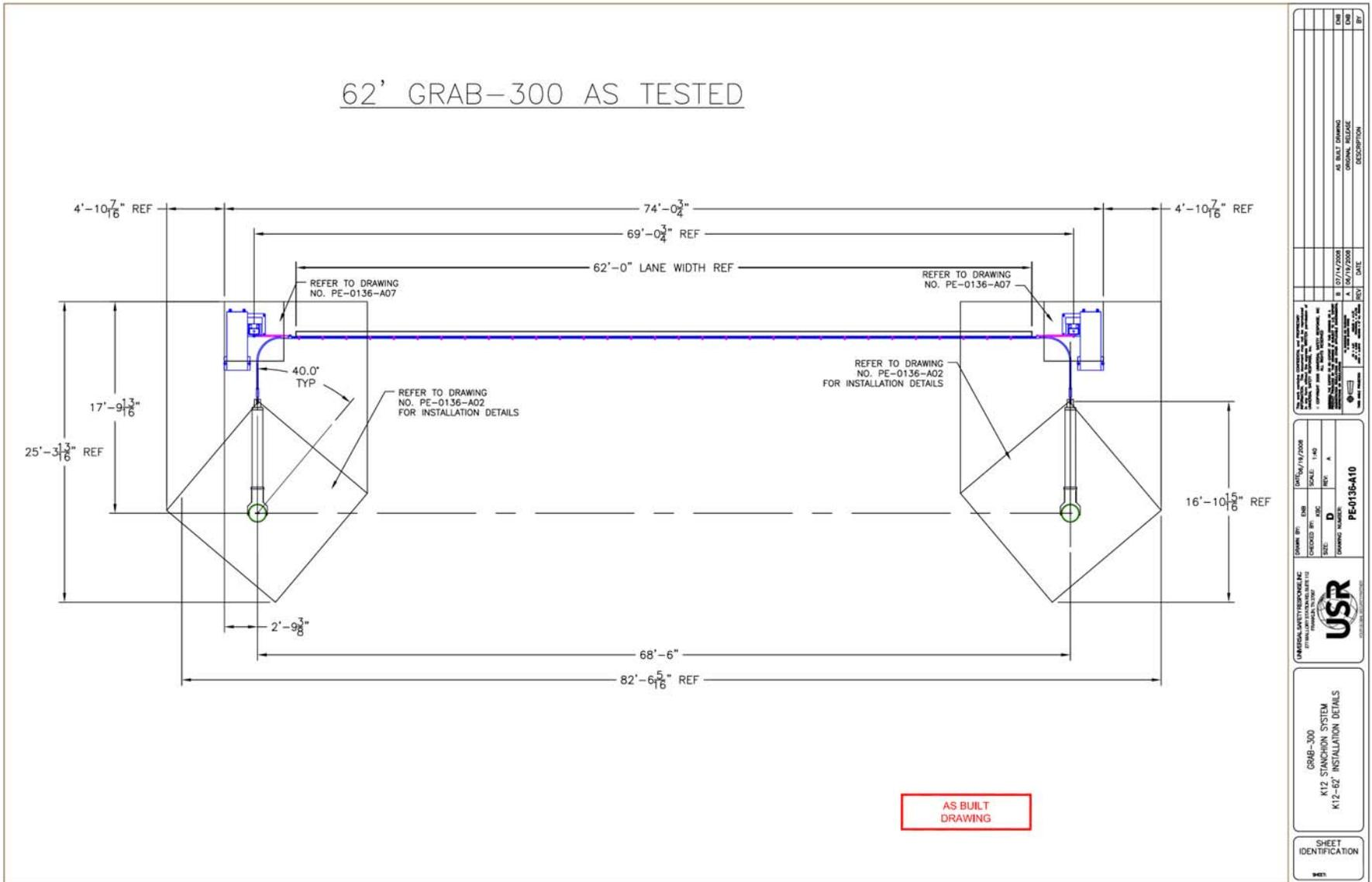
Figure 7. Details of the GRAB-300 62-ft barrier net – stanchion system installation details.
