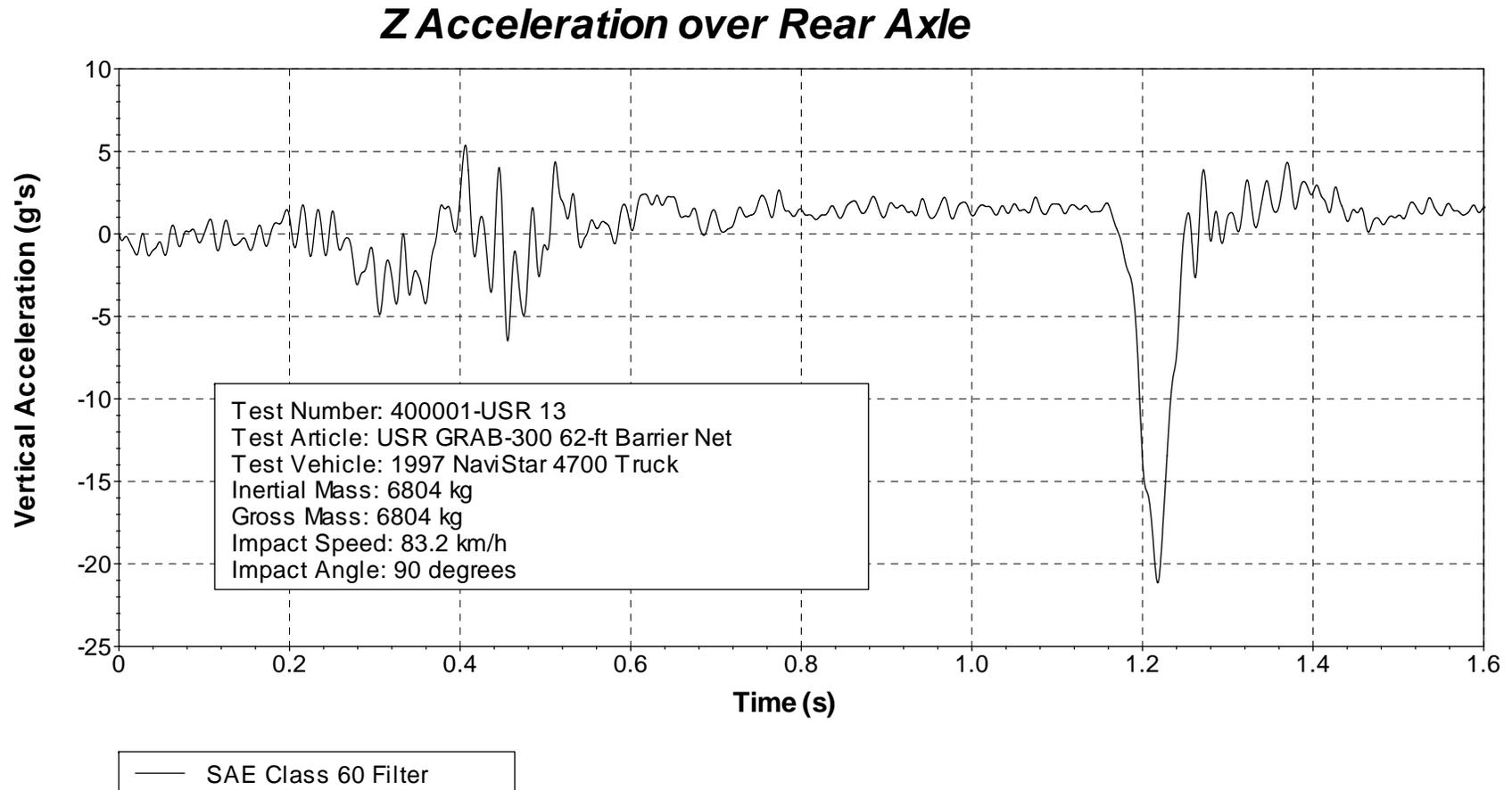
Figure 25. Vehicle vertical accelerometer trace for test 400001-USR13 (accelerometer located over rear axle).
