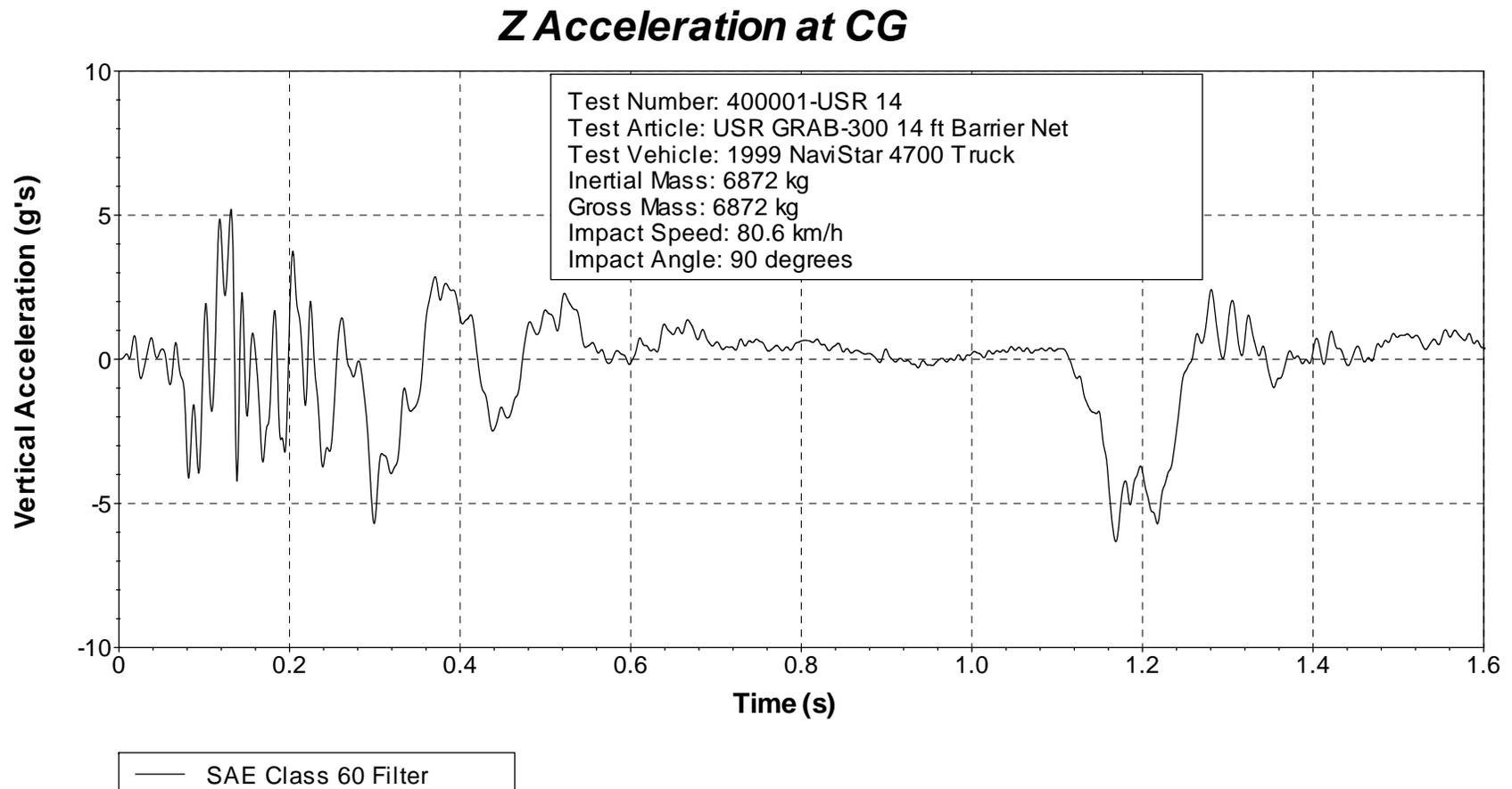
Figure 22. Vehicle vertical accelerometer trace for test 400001-USR14 (accelerometer located at center of gravity).
